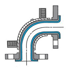
Ideal for circulating hot or cold liquid to control process conditions. Both inside and outside pipes are schedule 40 steel. Flanges are standard lap joint style as pictured below. Jacket can be extended to the flange, if required.
